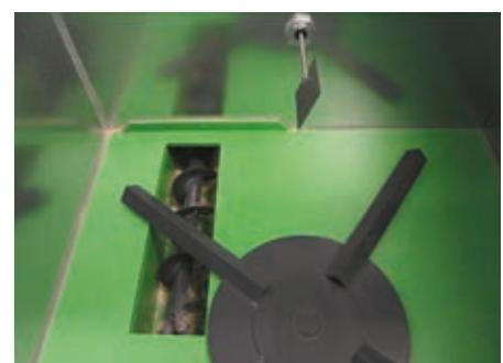
The continually turning tube extractor mixes the material and sends it to the discharge screw conveyor, which feeds it cyclically to the pressing mechanism.
