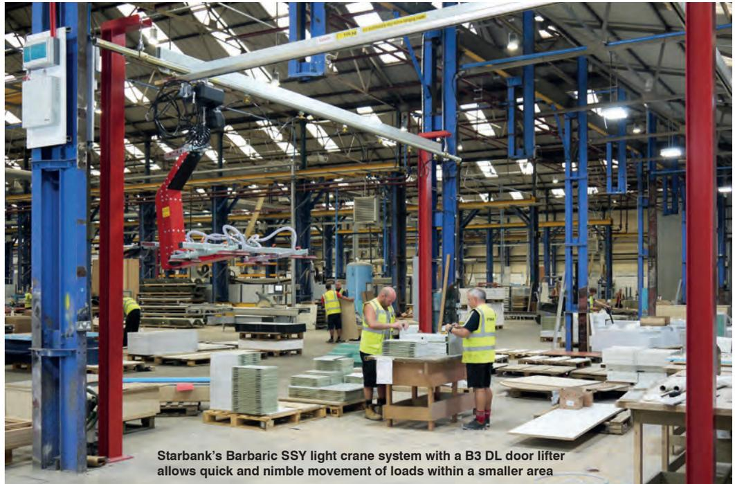
Starbank's Barbaric SSK light crane system with a B3 DL door lifter allows quick and nimble movement of loads within a smaller area
