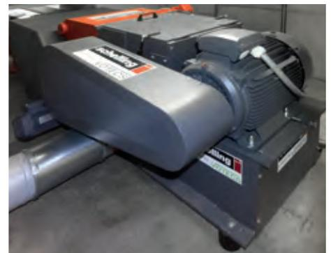
and the operators used to stack the pieces before shredding, but with the longer pieces it would have meant operators breaking them up and feeding them in. The new Votecs has a five-metre, vibrating channel that handles the three metre offcuts easily.” The operator throws them into the channel and the vibration feeds them into the machine automatically.
